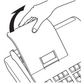
**2** Remove the battery compartment cover.
